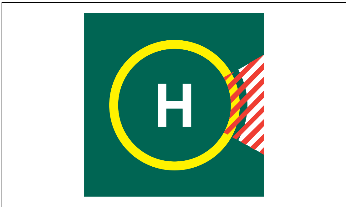
Figure 6 Example of Prohibited Landing Heading Marking
